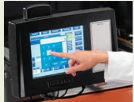
> A large 10.4-inch LCD color touch screen makes fonts easier to read for faster operation.
